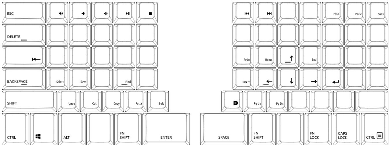
The Function Layout, indicated by blue characters, is activated by either pressing and holding the FN Shift key, or the activation of the FN Lock key. This layout activates:
