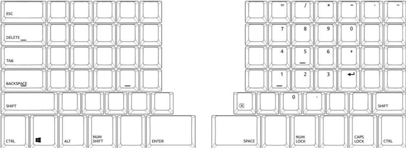
The NUM Layout, indicated by yellow characters, activates a standard Numpad layout. This is integrated on the right half of the keyboard. The layout is activated by either pressing and holding the NUM Shift, or by activating the NUM Lock key.
