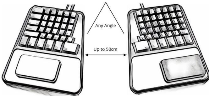
The split design of the keyboard allows for a distance between the halves of up to 50cm. You can set the distance between the two halves that suit you. One suitable position is to separate the boards to shoulder width.
