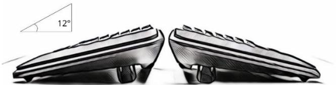
The tented angle can be increased to 12 degrees by extending the inner feet. This will further help to relieve pronation stress.
