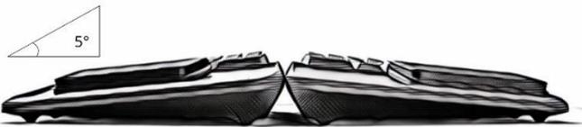
The tented angle of the default flat position is 5 degrees away from the center. This seemingly slight angle will make a noticeable difference in improving wrist stresses associated with pronation.
