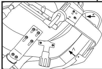
\*The cable of the lumbar goes under the bar of mechanism and back
