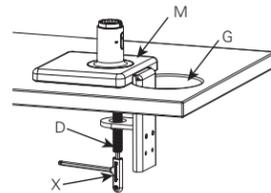
**NOTE:** If grommet hole is less than 3", the clamp will need to be separated as seen in step 1C.
