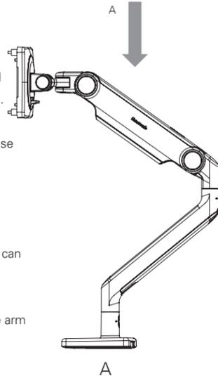
B. Adjust the screw with 4mm Key clockwise direction (towards +) to increase load tension and anticlockwise (towards -) to reduce load tension.
