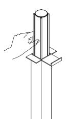
Step 2 Remove the cap from pole using a flat screwdriver
