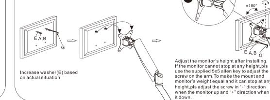
To adjust the monitor with the supplied 5x5 allen key(G)
