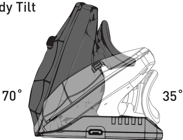
Hold base with one hand and top section with other hand. Tilt top section to set angle.
