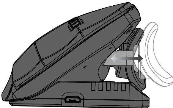
Hold thumb ext. between thumb and index finger, push and pull to set thumb width.
