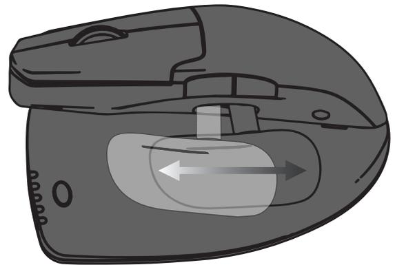
Hold thumb rest between thumb and index finger. Move rest horizontally to set desired position.
