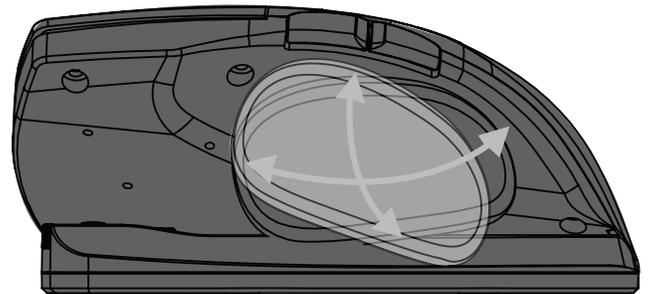
Place thumb on thumb rest. With slight pressure, rotate thumb to set desired position.
